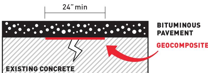
Clean and fill existing crack joint with approved hot poor sealant.
